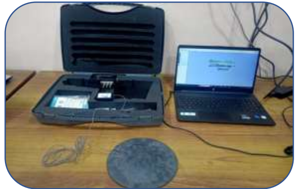
Triaxial Vibration Analyzer
